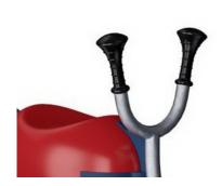
Handles are made with a moulded PP insert and an outer layer of soft TPV rubber. The handles are attached to the pipe with a galvanised steel inlay to ensure strength and durability.
