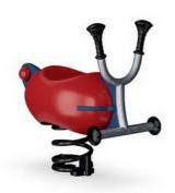
KOMPAN Springs are made of high quality spring steel according to EN10270. The springs are cleaned by phosphating before they are painted with an epoxy primer and a polyester powder coating as top finish. The springs are fixed by unique anti pinch fittings for maximum safety and long lifetime.
