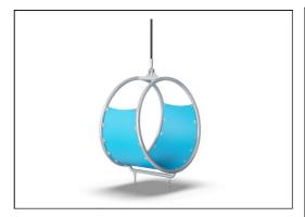
Hangout pod designed with a welded frame of two steel rings which are hot dip galvanized and powder coated. The membrane consist of friction-proof rubberized material of conveyor belt quality with excellent UV resistance. Max. fall height 8'9"
