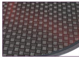
Deck plate of 3mm thick non skid aluminum or 17,8mm thick HPL plate. For warm locations KOMPAN recommends HPL deck plate as the aluminum will get hot in sunny conditions. Both deck plates ensures safe play for all users and is maintenance free.
