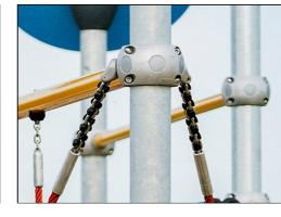
Corocord smart clamps are carefully designed in every detail to ensure superior flexibility in high quality aluminum material. The smart clamps are attached around the posts with four steel bolts. Not used attachment points are closed with PA caps.
