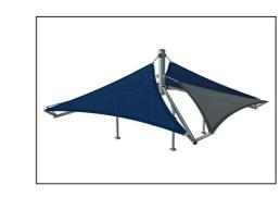
Sails of commercial 95 high-density PE knitted specially for sun-shade structures. The sails are treated with UV stabilisers to ensure longevity. The sails are supported by a hot-dip galvanised steel frame and tightened by stainless-steel devices.
