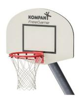
The basketball hoop is made from hot-dipped galvanized steel with a powder-coated finish. The net is made from Ø4 chain links made from S235 galvanized steel or stainless-steel chains, which meet the requirements in ISO1434-ISO1435 and DIN766. The chains have a circumference of ~Ø11.8in at the bottom and ~Ø19.6in at the top.
