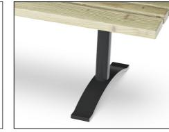
Powder coated top finish on top of galvanization is processed in two steps: Light grinding and clean sweeping, powder coating - thickness 70-120  $\mu m.$
