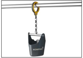
The sand bucket is made in one piece of molded PE. The PE is made with 33% post-consumer materials in different colors with a wall thickness of minimum 5mm. Material in accordance with the European Standard EN 71-3 and tested for UV stability.
