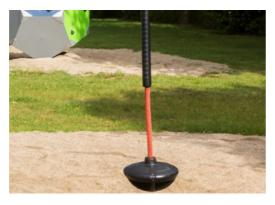
The special designed seat is made of a stainless-steel insert covered with a soft layer of PUR rubber. The seat is impact tested to fulfill all global playground standards and the rope has an ergonomic handhold of a 100cm long moulded on PUR rubber handle.
