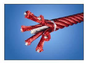
Corocord ropes with 19mm diameter or more are special 'Hercules' - type with galvanized six-stranded steel wires. Each strand is tightly wrapped with PES yarn, which is melted onto each individual strand. The ropes are highly wear-and vandalism-resistant and can be replaced at site if needed.
