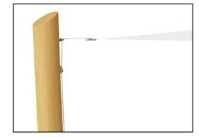
The rope is attached to the Robinia post by a stainless-steel eyebolt and tightened by a nylon bracket with wedge track. The system ensures the sail is easy to set-up, tighten and take down again.
