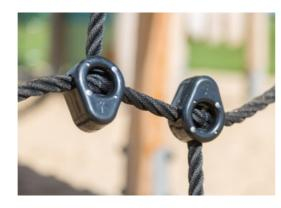
Ropes of UV-stabilized PES rope strands with inner steel cable reinforcement. The polyester yarn is made from +95% post-consumer materials and is inductively melted onto each strand. The stainless-steel slides with one-piece slide bed are made of high-quality stainless-steel AISI 304.
