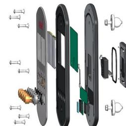
Front panels are made of UV-stabilized Polycarbonate. The UV-stabilization prevents the Transparent panels in being yellow over time and ensures the mechanical performances. The graphic prints are added by a unique multi-layer print process where the inner layer is the image and outer transparent layer functions as protection. The lacquer is water-based, and UV stabilized to prevent fading.
