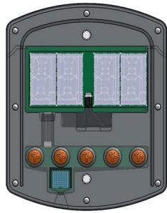
The reflective LCD display has four digits of 100mm height, with excellent outdoor visibility and a wide viewing angle. An LCD display has a low energy consumption, It is powered by 8 replaceable AA batteries with a lifespan of more than 2 years.
