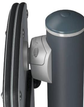
The connectors are made of die-cast aluminum specially alloyed for outdoor environments and with a lead content below 100ppm. The connectors are attached to the posts by stainless steel screws and well protected against corrosion by special designed zinc washers. Extremely strong and no chance of corrosion.
