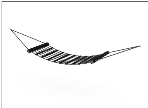
Hammock is made of steel reinforced single braided 16 mm UV-stabilized PES rope strands. The polyester yarn is made from +95% post-consumer materials and is inductively melted onto each strand. PES has high strength with excellent resistance to abrasion and UV radiation. The rope loops are connected by nylon (PA6) connectors providing a smooth and comfortable hammock.
