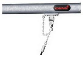
KOMPAN's swing hangers are heavy-duty and designed with stainless steel and anti-twist functions. The hangers attach to the cross beam on a welded bracket with two bolts. The bearings are embedded with silicone lubricant and need no further lubrication; ensuring low maintenance.
