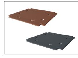
Floors and panel activities are available in two types of material: Waterproof plywood decks thickness 21.5mm from pine and alder wood with anti-slip film on both sides. High Pressure Laminate HPL thickness 17.8mm with slip resistant surface texture according to EN 438-6.
