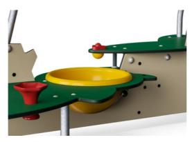
Yellow basin is made from UV-stabilised PC with a thickness of 3 mm. The basin can be lifted up for emptying. The basin is fixed to the structure by a steel chain to prevent removal.
