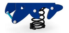
KOMPAN Springs are made of high quality spring steel according to EN10270. The springs are cleaned by phosphating before they are painted with an epoxy primer and a polyester powder coating as top finish. The springs are fixed by unique anti pinch fittings for maximum safety and long lifetime.
