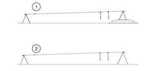
KOMPAN cableways are available for flat or natural sloped surroundings and for surface or in-ground installation. Further the cableways can be supplied with one or two cables for children to ride together in friendly competition. For flat surroundings a starting mound or platform is needed to use the cableway.
