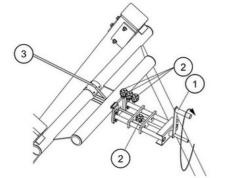
The steel cable 3 is tensioned by a special designed device. By turning the handle 1 the steel cable can be tensioned according to instruction in a safe way. After tensioning the cable is locked by three clamps 2. The tensioning device can also be used for adjustment during annual inspections.
