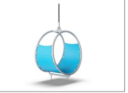
Installation Information Max. fall height 152 cm Safety surfacing area 59.8 m<sup>2</sup> Total installation time 20.5 Excavation volume 1.48 m<sup>3</sup> Concrete volume 0.04 m<sup>3</sup> Footing depth (standard) 90 cm Shipment weight 570 kg Anchoring options In-ground Surface **Warranty Information** Galvanised/painted 10 years metal Hot dip galvanised steel Lifetime Polycarbonate PC 10 years panels PUR components 10 years Spare parts guaranteed 10 years
