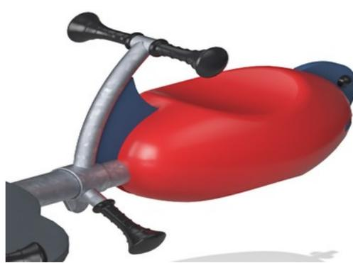
Handles and footrests are made with a molded PP insert and an outer layer of soft TPV rubber. The handles and footrests are attached to the pipe with a galvanized steel inlay to ensure strength and durability.
