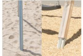
The post of the A-Frame swings are available for surface anchoring with expansion bolts or inground in 60cm or 90cm depth. The hot dip galvanised steel legs are anchored directly in the ground. Pine wood posts are elevated from ground by a unique profiled hot dip galvanised steel footing.
