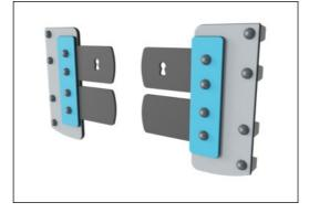
Membranes consist of friction-proof rubberized material of conveyor belt quality with excellent UV resistance. Embedded is a four-layered armouring made of woven polyester. The armouring and the two surface layers result in a total thickness of 9 mm.
