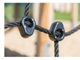
Nets and ropes are made of UV-stabilised PA with inner steel cable reinforcement. The rope is induction treated in order to create a strong connection between steel and rope which leads to good wear resistance.
