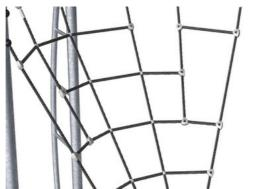
Climbing nets are made of UV-stabilised PA rope with inner steel cable reinforcement. The rope is induction treated to obtain maximum fixation between steel and rope which provides excellent wear and tear resistance. All rope connectors are made of 100% recyclable PA material.
