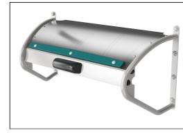
The curved start platforms are made of a curved stainless steel plate with non skid texture. The lower part of the platform is supported by a EcoCore board for safe foothold and the rubber bumper is placed to receive the pole.
