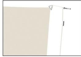
All fixation points are equipped with steel brackets to ensure strong connection to the nylon rope used for tightening.
