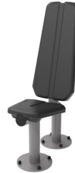
The seat and back support are made of Polyurethane Rubber (PUR) and have an electro-galvanized steel insert plate that connects the seat to the frame. The seat is positioned under a 9-degree angle and the back support has a 15-degree angle. The back support has a groove to relieve the spine, accommodating a comfortable seating position.
