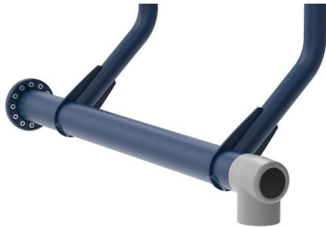
The input shaft is Ø101,3 x 2,9mm S355 Hot Dip Galvanized and Powder-coated steel. The bearing house is Cast Aluminum (EN AB-44100 / EN AB-AISI12(a)) with self-aligning sealed ball bearings. An extremely strong and durable construction.
