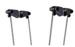
The double steel yoke suspension provides the unique parallel movement of the seat. The swing hangers are made of high-quality UV stabilised nylon (PA6) housing with integrated lifetime sealed ball bearings. The height-adjustable chains are fixed by a stainless steel hook with a theft-proof snake eye bolt in a turnable anti-twist housing.
