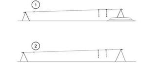
KOMPAN cableways are available for flat or natural sloped surroundings and for surface or in-ground installation. Further the cableways can be supplied with one or two cables for children to ride together in friendly competition. For flat surroundings a starting mound or platform is needed to use the cableway.
