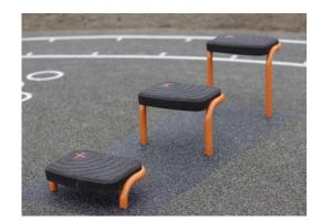
The support frame is ø48.3 x 4mm, carbon steel, with a hot-dip galvanised surface according to ISO1461, and a powder coating corrosion class C3 according to ISO12944-2. Lead content for surfaces are below 90ppm.
