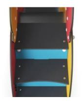
The steps are made of High Pressure Laminate HPL with a thickness 17,8mm and non skid surface texture according to EN 438-6. KOMPAN HPL has high wearing strength to ensure long lifetime in all climates.
