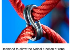
play structures to move Corocord 'S' clamps are used as universal connections in Corocord products. 8mm stainless steel rods with rounded edges are pressed around the ropes with a special hydraulic press, making them the ideal connector. Our clamps are safe, durable and vandalism-proof.
