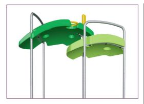
The ELEMENTS roofs are made of recyclable PE with a minimum wall thickness of 5 mm to ensure high durability in all climates around the world. The steel pipes are hot-dip galvanised inside and outside for maximum durability.
