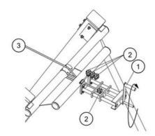
The steel cable 3 is tensioned by a special designed device. By turning the handle 1 the steel cable can be tensioned according to instruction in a safe way. After tensioning the cable is locked by three clamps 2. The tensioning device can also be used for adjustment during annual inspections.
