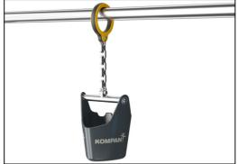
The sand bucket is made in one piece of molded PE. The PE is made with 33% post-consumer materials in different colors with a wall thickness of minimum 5mm. Material in accordance with the European Standard EN 71-3 and tested for UV stability.
