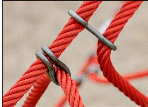
Corocord 'S' clamps are used as universal connections in Corocord products. 8mm stainless steel rods with rounded edges are pressed around the ropes with a special hydraulic press, making them the ideal connector: safe, durable and vandalism-proof, all while allowing the typical movement of rope structures.
