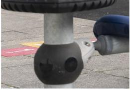
The hang-on puller is designed with at welded steel core and covered with low-density PE housing. The two rubber coated handles are angled to provide best possible ergonomic while gliding. The wheels of the puller are made of low noise TPU and installed with sealed ball bearings.
