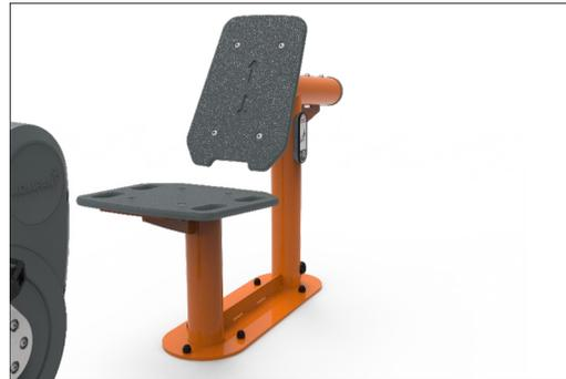
The seat and backrest is be made of Ekogrip™ panel that consist of a 15mm thick PE base with 3 mm top-layer of soft rubber with a non-skid effect. The backrest is adjustable, and the user can choose between 6 different distances to the bike.
