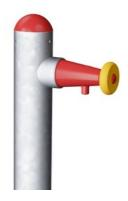
The steel surfaces are hot-dip galvanized inside and outside with lead-free zinc. The galvanization has excellent corrosion resistance in outside environments and requires minimal maintenance. The integrated water tap open for water when pushed and stops when letting go. The water is supplied trough a pipe located inside the post with hose or pipe connection at the bottom of the post. The supply can either be a loose hose or a permanent in-ground pluming.
