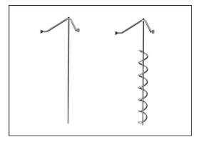
The stainless steel activities are made of high quality stainless steel. The steel is glass blasted after manufacturing to ensure a smooth gliding surface.
