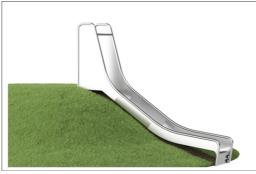
The stainless steel components are made of high-quality stainless steel in compliance with global playground standards. The steel is glass blasted after manufacturing to ensure a smooth gliding surface. At 35°, the slide is set to the optimum angle to ensure children experience thrilling slides while maintaining safety. Catering to different terrains, the embankment slides are available in 9 lengths ranging from 1 - 3 meters.
