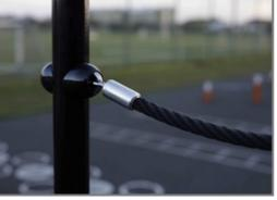
Ropes are made of UV-stabilised PES with inner steel cable reinforcement. The polyester yarn is made from +95% post-consumer materials and is inductively melted onto each strand, leading to good wear resistance.
