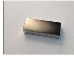
The magnets which are used are High Strength Neodymium magnets. The magnetic radiation is under strict control, the radiation level never exceeds 5 Gauss (0.5mT), which makes them perfectly safe to use as an training item.
