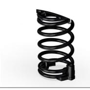
KOMPAN Springs are made of high quality spring steel according to EN10270. The springs are cleaned by phosphating before they are painted with an epoxy primer and a polyester powder coating as top finish. The springs are fixed by unique anti pinch fittings for maximum safety and long lifetime.
