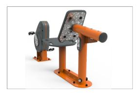
To ensure the integrity of the machine, the orange-colored main posts are made of ø101.6 x 3mm s235 steel posts, which are hot dip galvanized and powder coated.
