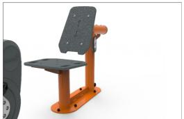
The seat and backrest is be made of Ekogrip™ panel that consist of a 15mm thick PE base with 3 mm top-layer of soft rubber with a non-skid effect. The backrest is adjustable, and the user can choose between 6 different distances to the bike.
