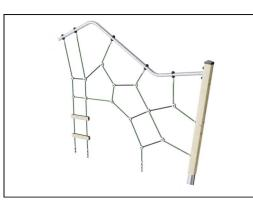
Corocord ropes of UV-stabilized PES rope strands with inner steel cable reinforcement. The polyester yarn is made from +95% postconsumer materials and is inductively melted onto each strand. PES has high strength with excellent resistance to abrasion and UV radiation. The rope loops are assembled by aluminum connectors.
