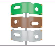
The climbing elements displayed are moulded from 33% post-consumer recycled materials in one piece, with a minimum 5mm wall thickness. The climbing elements are made of recyclable PE which has a high impact resistance across a wide temperature span which ensures vandal resistance in all locations.
