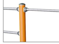
All bars intended for pull ups are made of solid, ø32mm x 138 m, hot dip galvanised, S235JR steel bars. This diameter gives the right grip for everyone.
