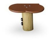
The steps are made of 21,5mm thick plywood made from alder and pine wood. Both sides are covered by 2 layers of phenolic film with anti slip net pattern. All cutting edges are sealed with paint to ensure long lifetime.
