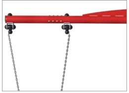
The seat hangers are made of high-quality UVstabilised nylon (PA6) housing with integrated lifetime sealed ball bearings. The chains are fixed by a stainless steel hook with theft-proof snake-eye bolt in a turnable anti-twist housing.
