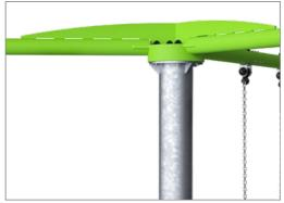
Center post is hot-dip galvanised in dimension Ø159 x 4 mm. Horizontal beams are hot-dip galvanised and powder coated in dimension of Ø76.1 x 3.6 mm.
